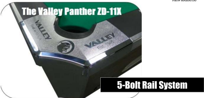
Besides having 5 attachment points, cushion rails are now secured with threaded inserts instead of T-nuts. This eliminates the small dead spots some players noticed at the rail bolt attachment points, makes the rails less susceptible to breakage and cross-threading, makes the rails easier to repair if an insert should require replacement – and they still fit 3-bolt tables 1970-1999
