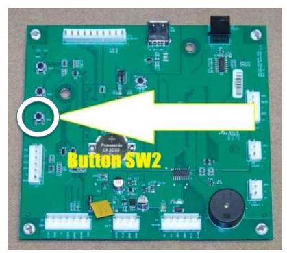
To begin programming, open the table's DBA Coin door and locate button "SW2" on the main PCB
