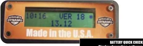
Display shows time, software version **Battery voltage** At 13.12v this table's battery is sufficiently charged
