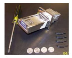
1) Remove the Push Chute from the coin door and – for easier access-remove the push chute end or anything bolted to the end. You will need the Push Chute (of course), enough coins or tokens to make it work in its current setting, the inserts for the desired setting, and a Phillips screwdriver.
