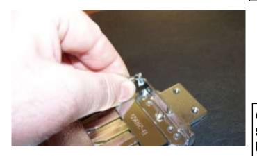
4) and unhook the two large return springs from the small hooks on the spring bracket.
