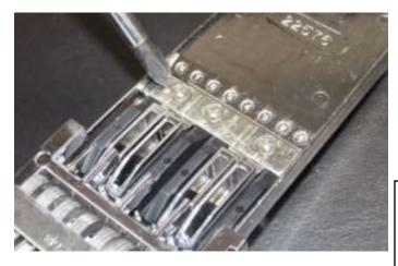
6) Remove the Phillips screw or screws holding the insert retainer plate and you will have access to all the inserts.
