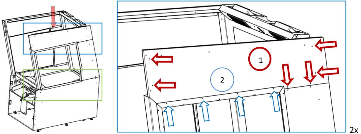
**8) Install the lower bolts for the window assembly**
