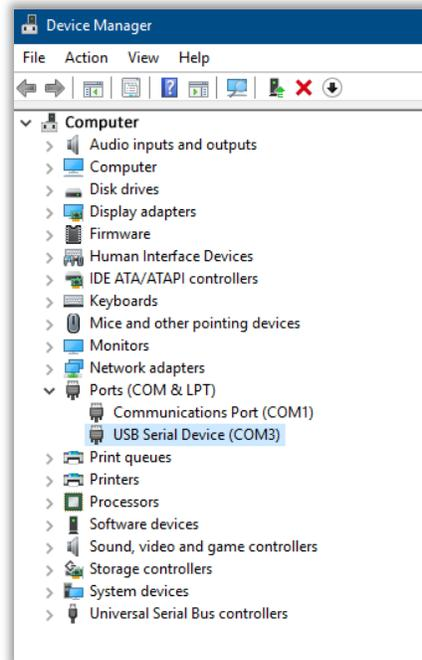
Verify that the “USB Serial Device” is set between COM2 to COM9.
