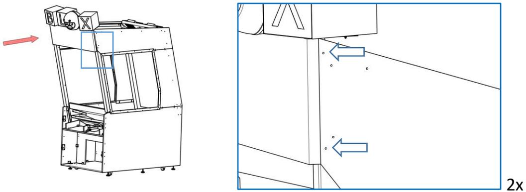
**11)** Install the ceiling light platform by sliding it from the back of the machine
