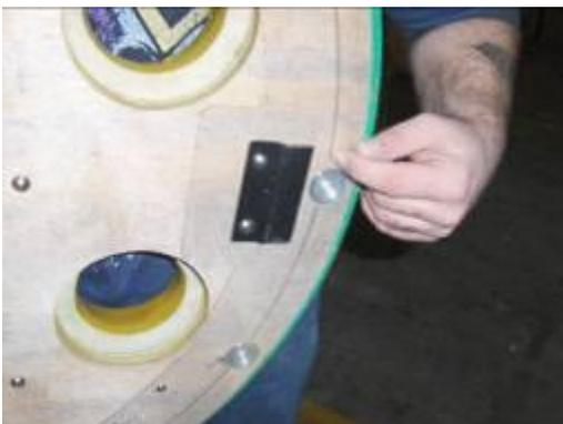
11. Remove 4 bolts to the mole head assembly. ( 1 in each corner).
