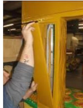
7. Unplug the ribbon cable and carefully pull the ribbon cable and wires up through the tower.
