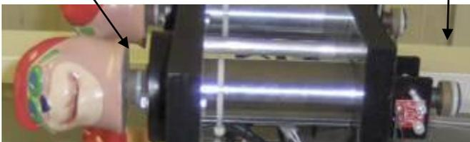
Clean the shaft using a soft cloth and an electrical contact / anti corrosion cleaner such as ElectriCorr VPCL – 239 or equivalent.
