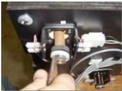
16. Remove Mole Head from the Assembly by pulling it out and then remove the 3 washers from the shaft.
