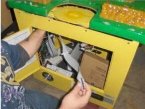
10. Carefully lift the top of the play field and unplug the molex connector.
