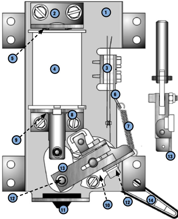
Figure 5.11.1. Left flipper assembly 500-6543-02-ND bottom view.
