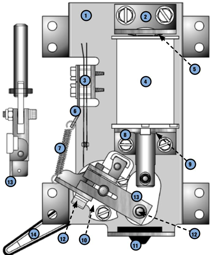
Figure 5.12.1. Right flipper assembly 500-6543-12-ND bottom view.
