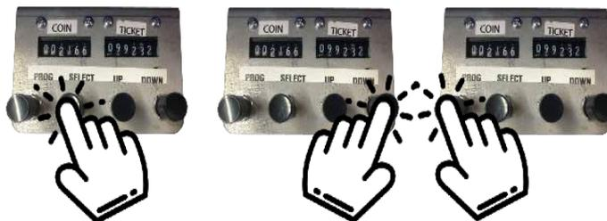
Press the “SELECT” button to enter the clear audit menu. Then change the value to 1 by pressing ‘UP’ or “DOWN” buttons. Press the “PROG” button if finished. Audits will not clear until you press the “PROG” button.
