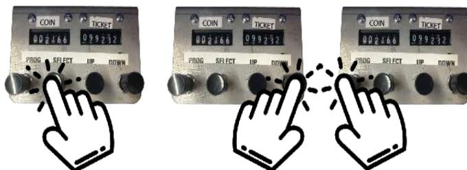
Press the “SELECT” button to enter the clear credits menu. Then change the value to 1 by pressing ‘UP’ or “DOWN” buttons. Press the “PROG” button if finished. Credits will not clear until you press the “PROG” button.
