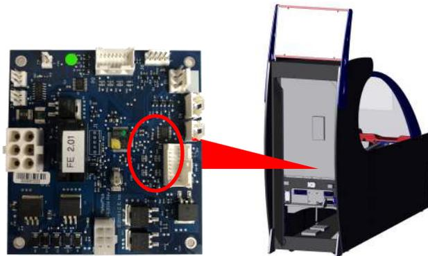
If all sensors fail self check, check harness the connection at P4 of I/O.
