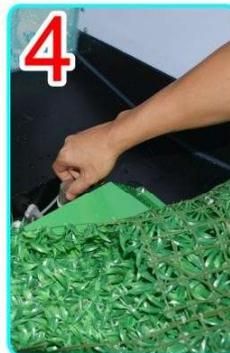
4 Rotate the filter out.
