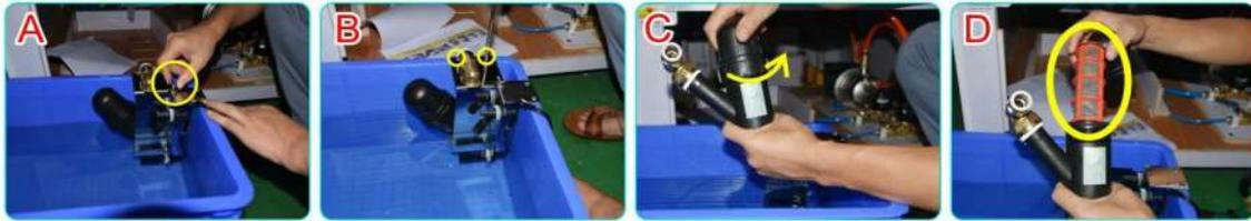
1. Unscrew the screw (as picture A), and unscrew the two small screws (as picture B) and then take out the filter.
