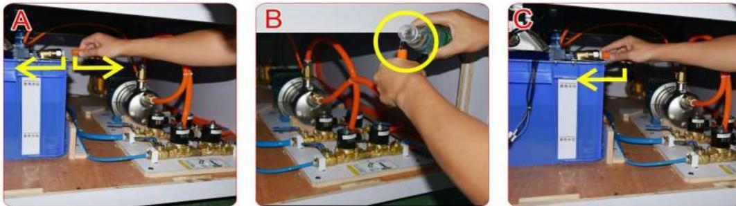
**because water pump is vacuum inside, please fill water into water pump before power on machine.**
