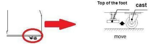
When moving the machine for a short distance, you should raise the foot to make the trundles touch the ground and push the machine.
