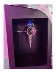
③ After adjustment, press the blue regulator cap down.
