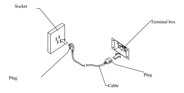
Warning: The working voltage of the machine is 220V. Please connect the power supply according to the label, or the machine might be damaged.
