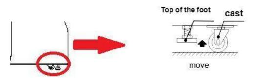
Please unplug the power socket before moving to prevent accidents and failure.
