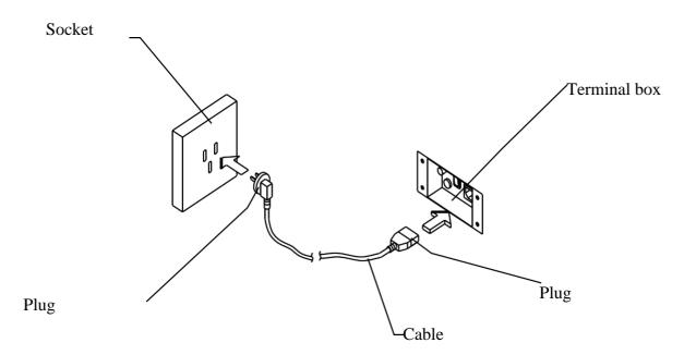
**Arning:** The working voltage of the machine is 110V in the USA. Please connect the power supply according to the label, or the machine might be damaged.
