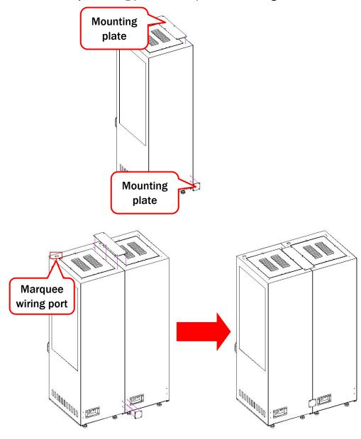
Step 7 Install Marquee. Utilize screws to secure. Connect the connectors.
