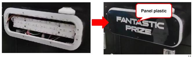
Step 6-1 First check and find Mounting plate on the machine back&top side. Loosen screws to remove Mounting plate.
