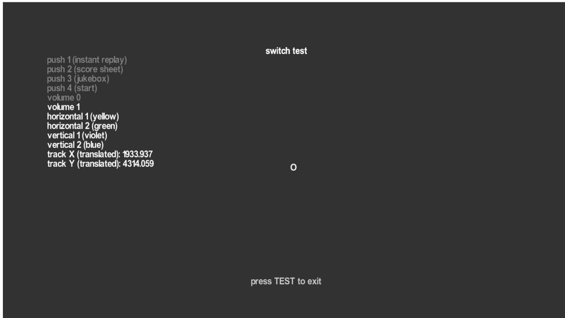
To assist in the diagnosis of trackball problems each of the trackball inputs are listed. Also, a count is shown for X and Y as the ball is spun.
