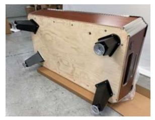
9. Screw the Leg Levelers all the way in and replace the Bottom Access Door.
