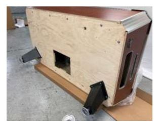
8. Attach each leg to the bottom of the table using 4 bolts. Attach the bottom two legs first.
